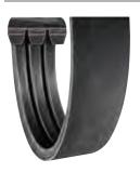
An excellent choice for narrow multiple drives where belt whip and turnover are a problem. The tie-band process assures smoother, trouble-free service. Banded belts are ideally suited for pulsating or heavily shock loaded drives and drives with long center distances.
