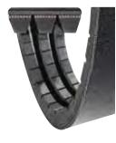
This is the banded version of the Power-Wedge Cog-Belt. It combines the superior flexing and controlled grip of the Power-Wedge v-belt with the qualities of a banded belt to minimize belt whip and turnover. The Power-Wedge Cog-Band also provides outstanding resistance to oil, heat and harsh environmental conditions.
