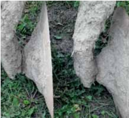
Typical picture of a compact disc harrow covered in dirt following the use of liquid manure.
